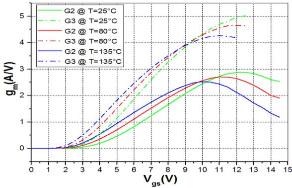
Fig. 4. Transconductance  $g_m$  as a function of  $V_{gs}$  at three temperatures (25°C, 80°C and 135°C) for two generations G2 (solid) and G3 (dashed).
