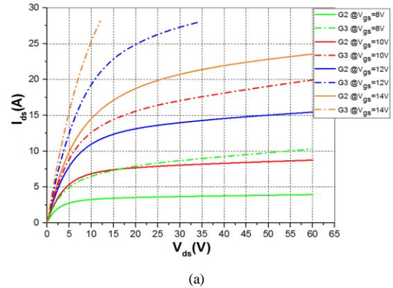
Fig. 3. Output characteristics for  $V_{gs}$  (8V, 10V, 12V and 14V), and for two generations G2 (solid) and G3 (dashed), at two temperatures: (a) 25°C, and (b) 135°C.
