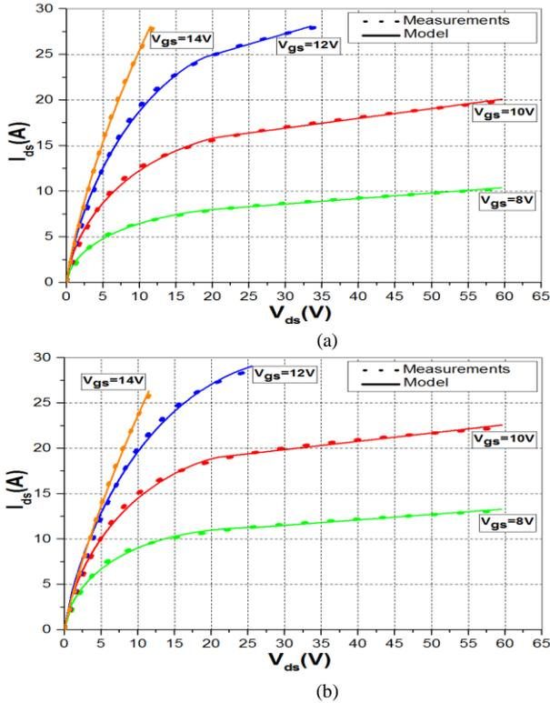
Fig. 9. Comparison of the output characteristics between the compact model and the measurements of the third generation of SiC MOSFET at two temperatures: (a) 25°C, and (b) 135°C.
