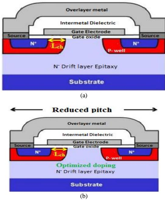
Fig. 1. MOSFET structure: (a) second generation (G2), and (b) third generation (G3) [17].
