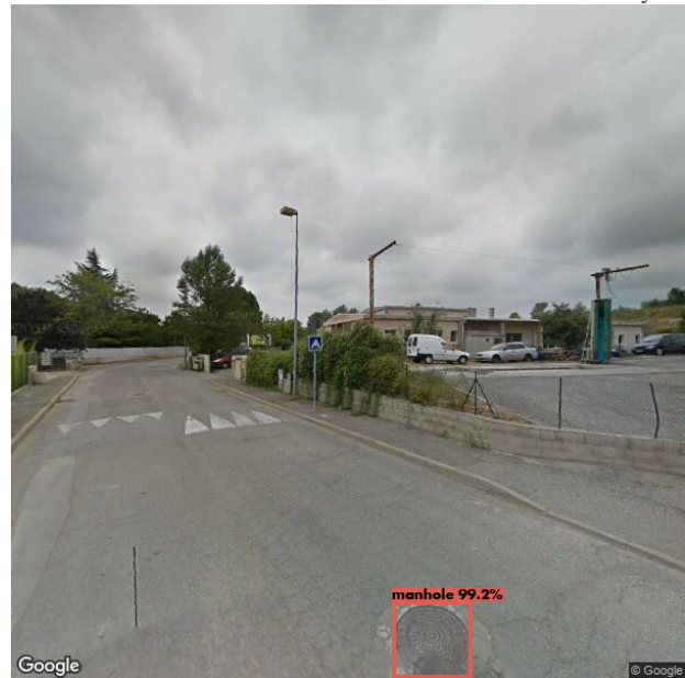
Fig. 12: Example of manhole covers' detection using Google Street View images
