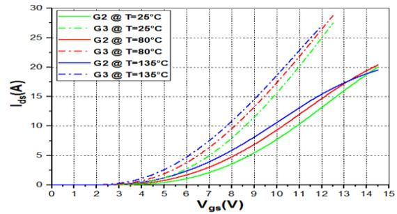
Fig. 2. Input characteristics for  $V_{ds}=18$  V, at three temperatures (25°C, 80°C and 135°C) for two generations G2 (solid) and G3 (dashed).
