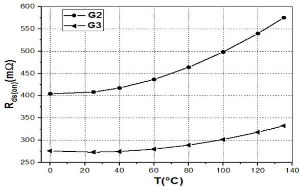
Fig. 5. On-state resistance  $R_{ds(on)}$  as function of temperatures at  $V_{ds} = 20V$  for two generations G2 and G3.
