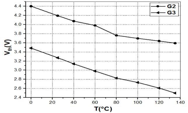
Fig. 10. Threshold voltage  $V_{th}$  as function of temperature at  $V_{ds}=20$  V for two generations G2 and G3.
