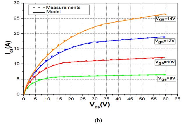
Fig. 8. Comparison of the output characteristics between the compact model and the measurements of the second generation of SiC MOSFET at two temperatures: (a) 25 °C, and (b) 135 °C.
